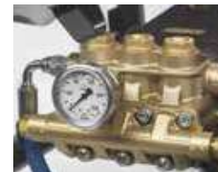
Comet TW-TW 500 Premium triplex pumps
