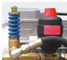
Unloader valve and pressure damper
