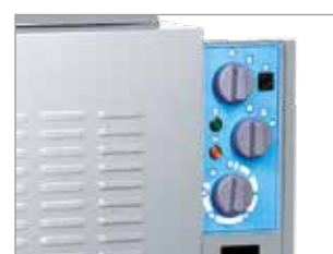
PILOT LIGHTS INDICATING MACHINE AND BURNER FUNCTIONING, PLUS FLAME CONTROL
