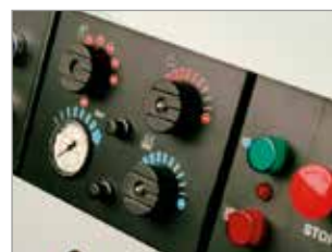
CONTROL PANEL PROVIDED WITH EMERGENCY SHUTDOWN
