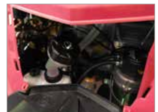
EASILY ACCESSIBLE ANTISCALE TANK
