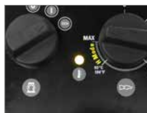
WARNING LAMP INFORMS WHEN TEMPERATURE IS BETWEEN 90-100°C
