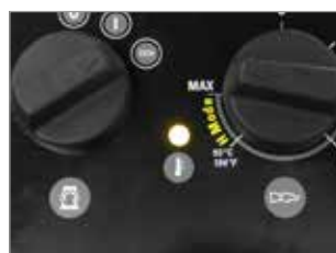
WARNING LAMP INFORMS WHEN TEMPERATURE IS BETWEEN 90-100°C
